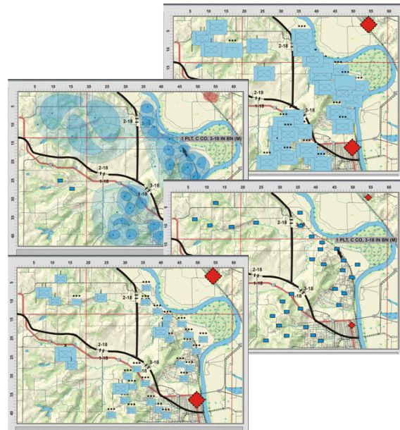
Figure 1. Display modalities investigated were (clockwise from top right) standard, miniature, proportional, and blobs.
